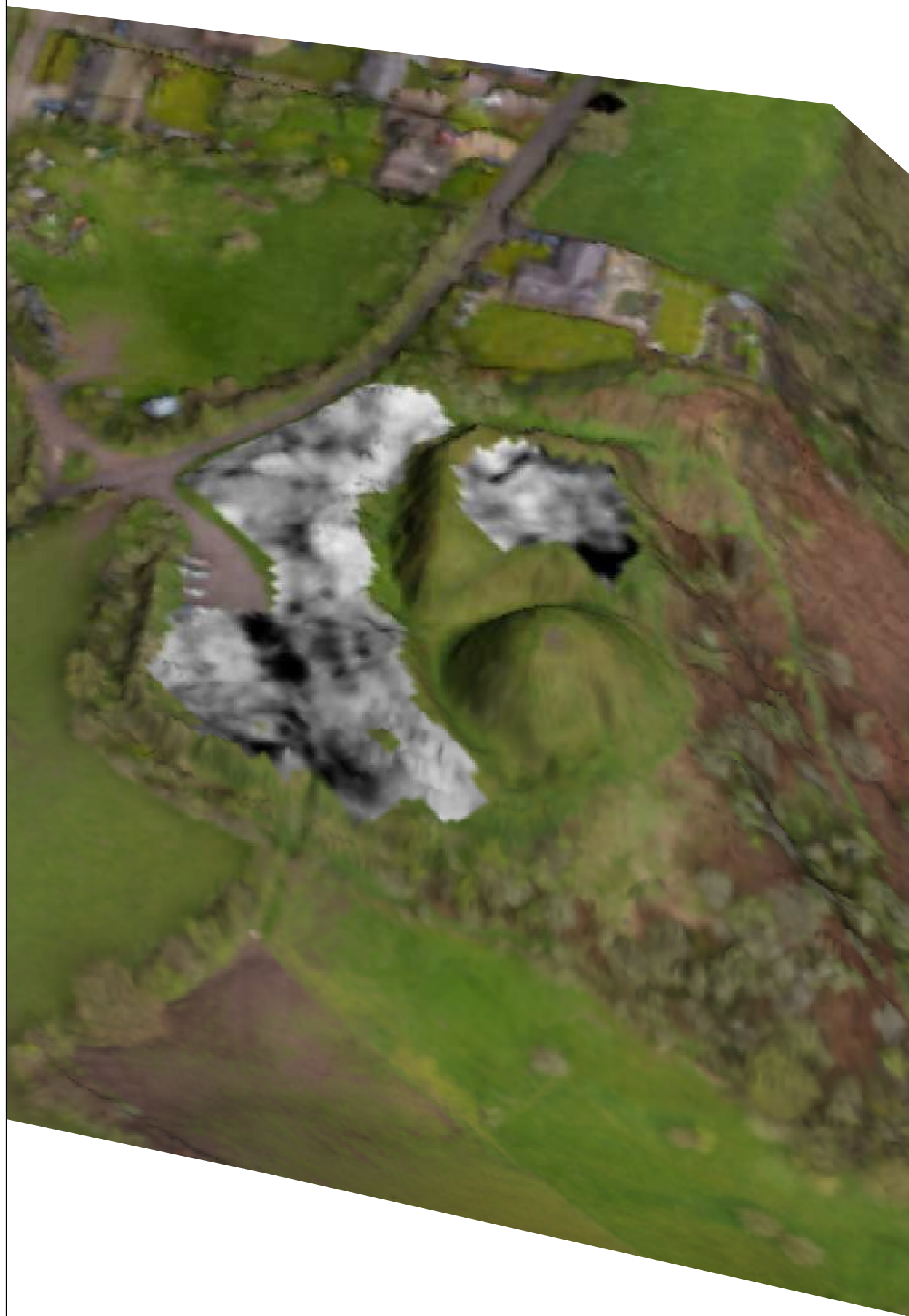
Surface overlay of aerial image over LiDAR DSM with resistivity greyscale
