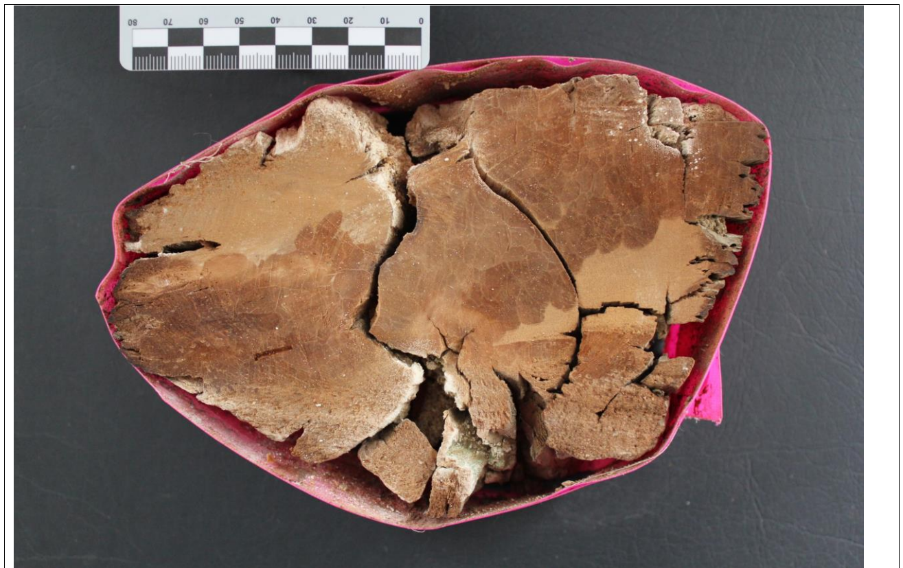
Figure 7 Castle of Old Wick slice sample CWK01 transverse section, as prepared by razoring for tree-ring width sequence measurement and for radiocarbon sub-sampling (see Table 1). Scale in 1cm blocks. Photo: C Mills.
