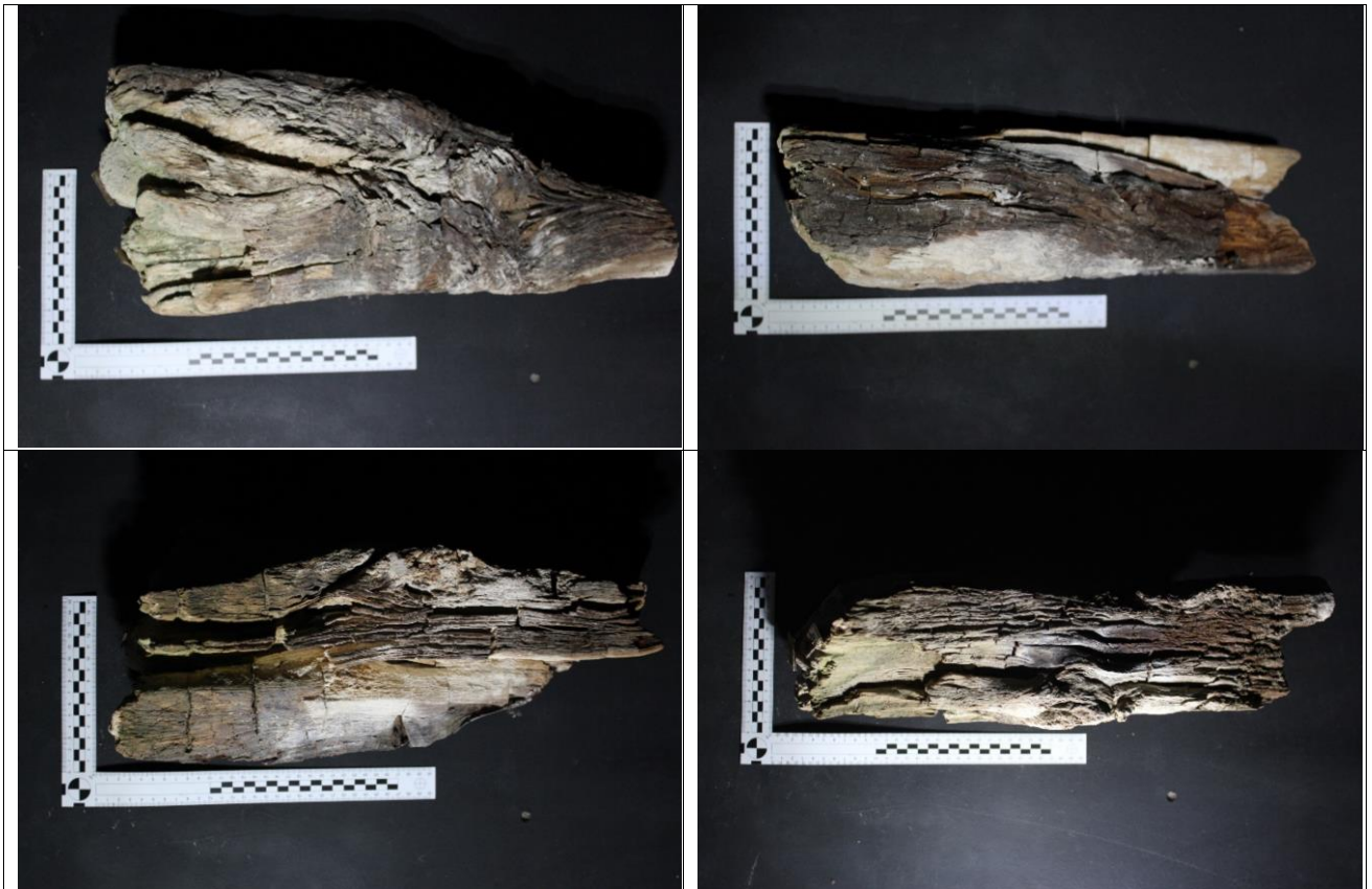
Figure 4: Record shots of the four side faces of the Castle of Old Wick timber. Black and white grid on scale is at 1cm intervals. Photos: Hamish Darrah 30.09.21.
