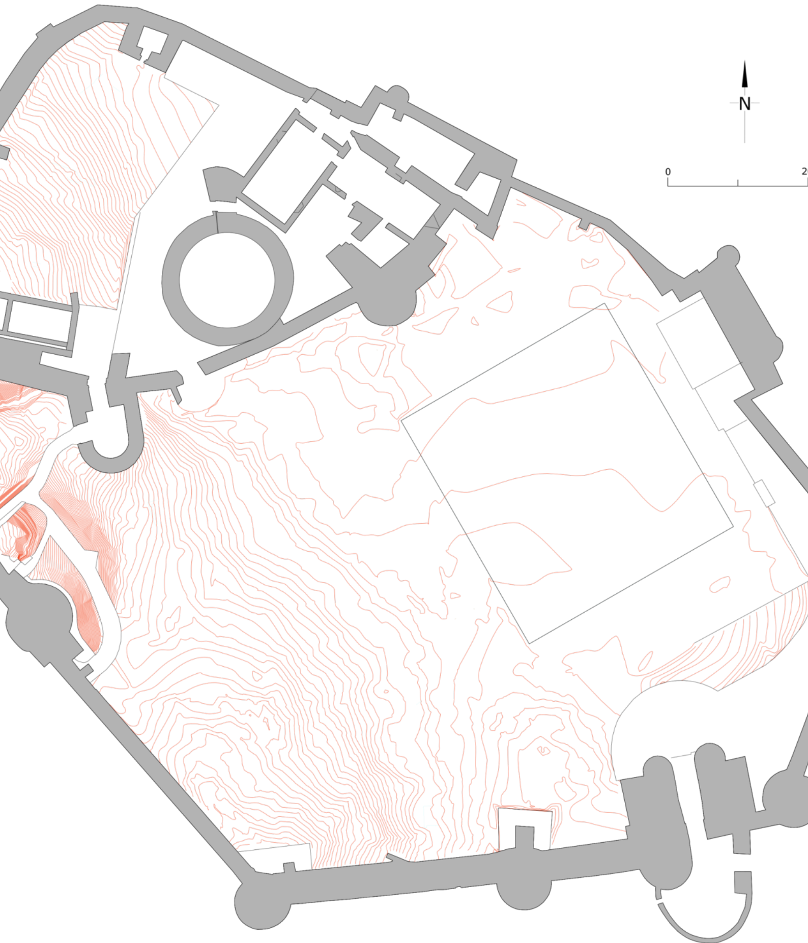
General contour plot from topographic survey with all internal walls of the castle surveyed supplemented with existing data (Ordnance Survey) where survey was not possible around the perimeter or for widths of some walls
